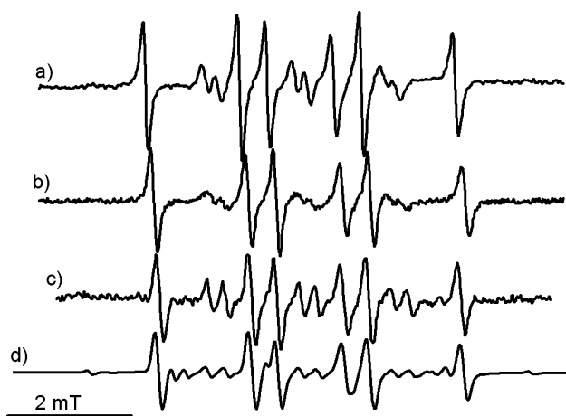
Figure 3. EPR spectra of various nitroxides derived from T-PBN: (a) signal recorded from the supernatant of a saturated aqueous T-PBN solution; (b) signal recorded after generating \cdot\text{OH} using a standard Fenton system in the presence of 0.008 mol·L -1 T-PBN in phosphate buffer; (c) signal recorded after generating \cdot\text{CH}_3 using a standard Fenton system in phosphate buffer/DMSO (80/20) in the presence of 0.008 mol·L -1 T-PBN; (d) signal recorded after generating \cdot\text{CH}_3 using a concentrated Fenton system in phosphate buffer/DMSO (80/20) in the presence of 0.15 mol·L -1 T-PBN.
